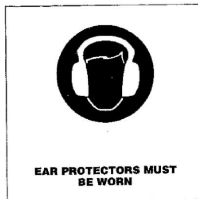
A: Sign for informing that ear protectors should be worn. (white on a circular blue background) Based on BS 5378 Part 1:1980
